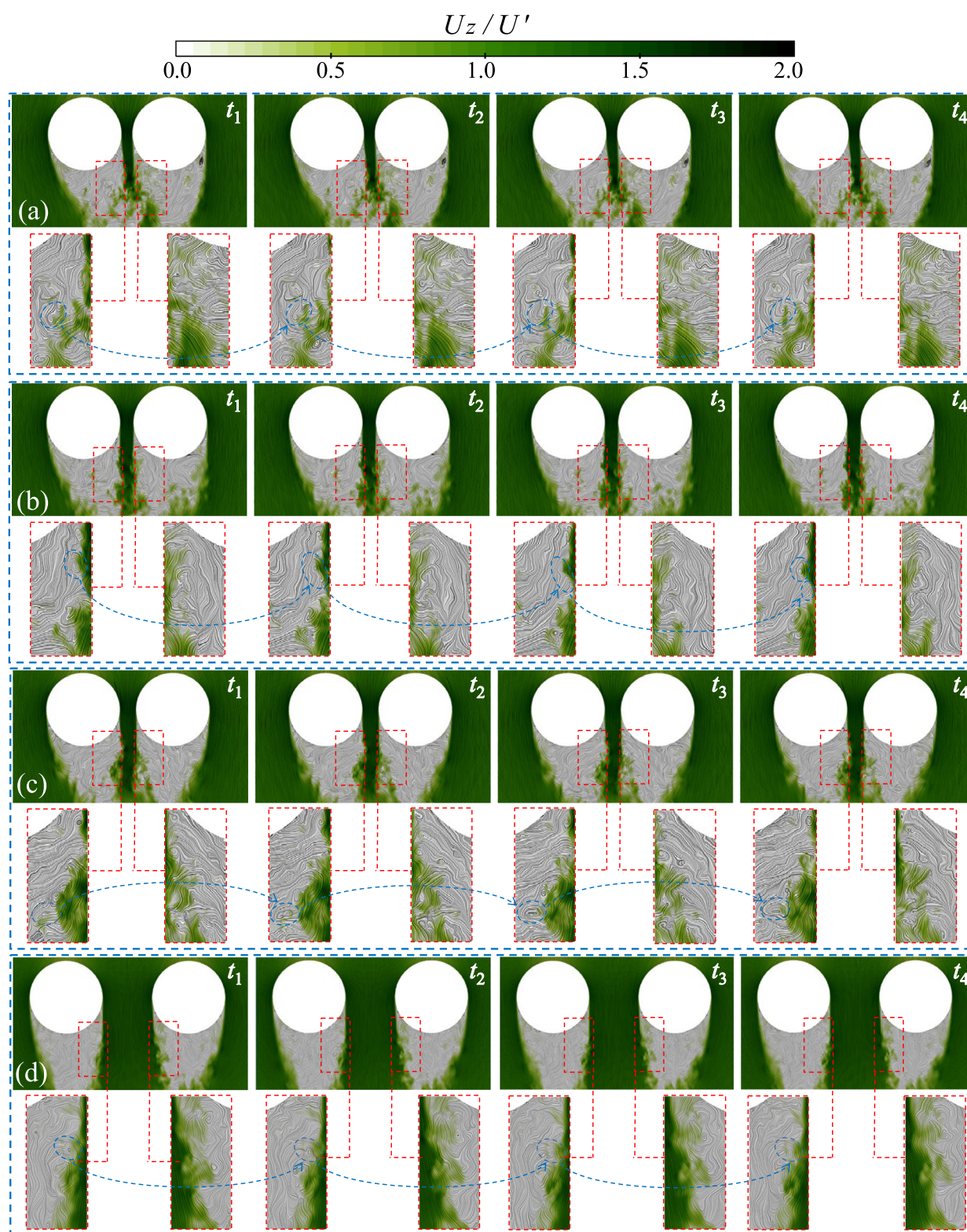
FIG. 21. The evolution of vortex structure on the horizontal profile at a height of 0.2H' in the gorge: (a) GM-0 ; (b) GM-0.5 ; (c) GM-1 ; and (d) GM-7 .
