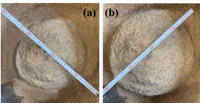
FIG. 8. Slurry injection of a crystalline body in a saturated sand layer: (a) Without considering slurry replacement and (b) considering slurry replacement.
