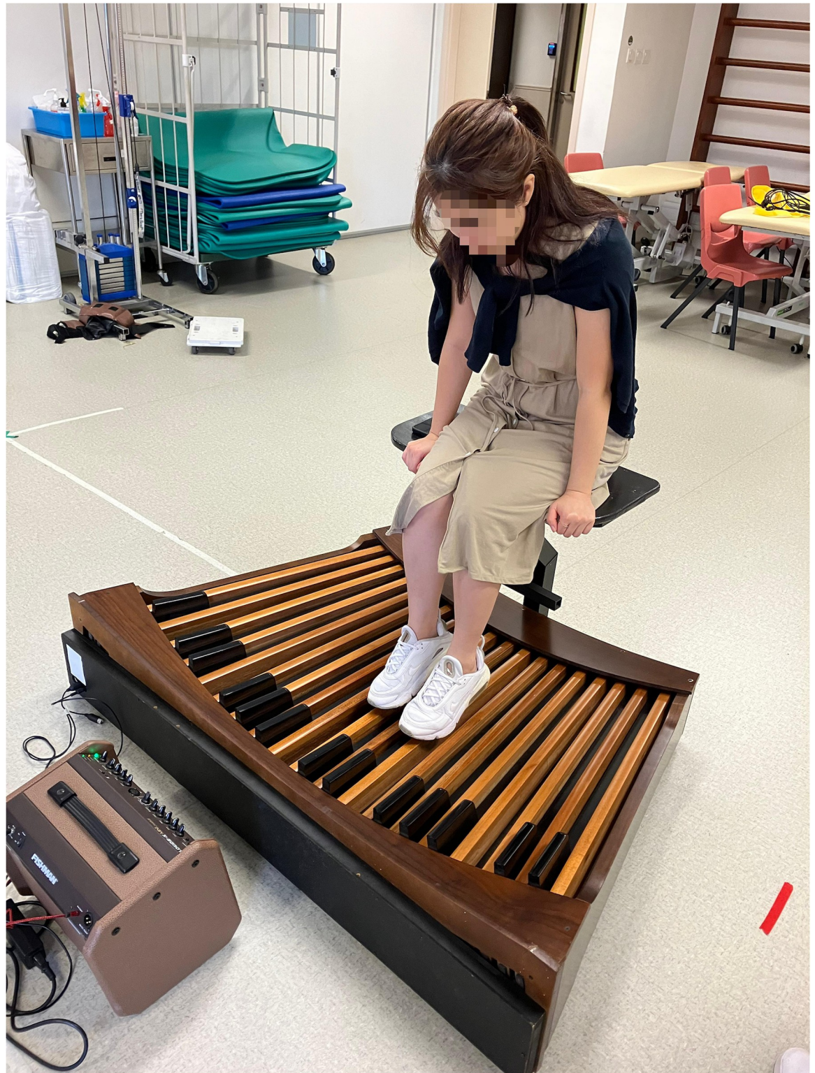
Fig 1. The modified pedalboard with a MIDI function.
