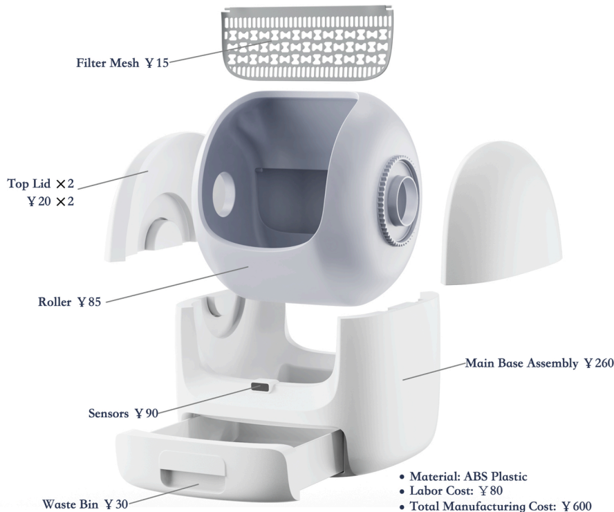
Fig. 16. Exploded-view drawing with cost estimation for the proposed product ideation.
