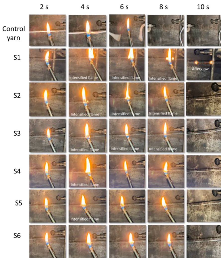
Fig. 5. Testing the flammability of control and oxidised acrylic yarns after 10 s in contact with flame.
