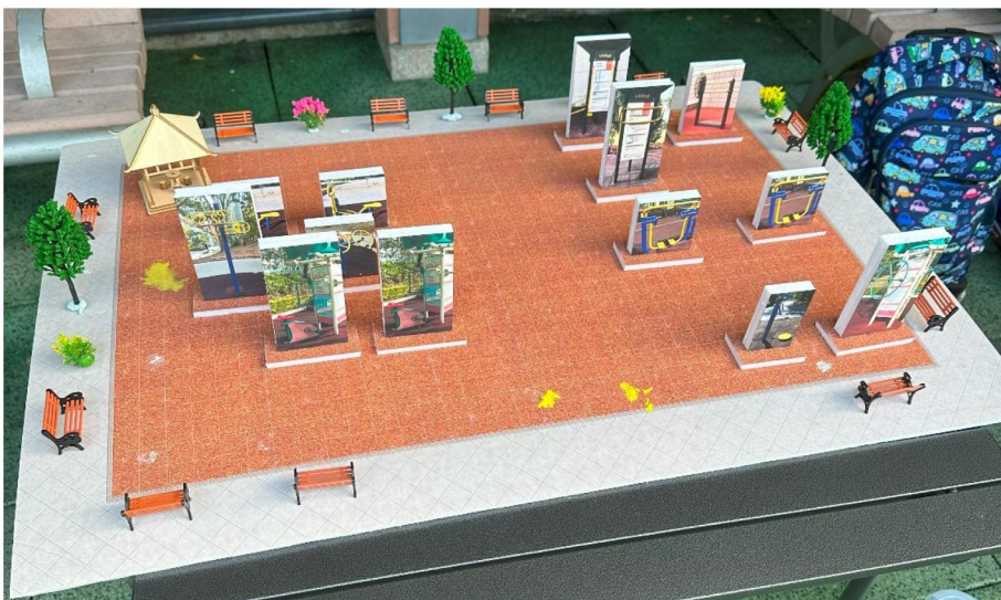
Figure 2. Selected senior-friendly outdoor gym model illustrating that exercise apparatus should be spaced out in a way that reflects the dynamism of exercise movement.
