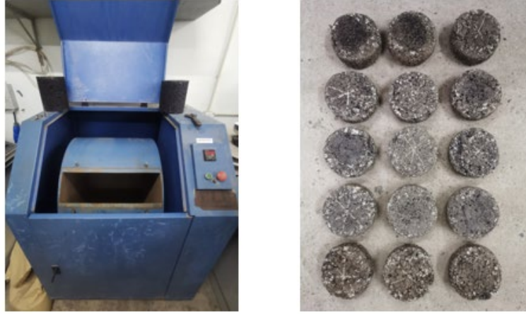
192 193 194 Fig. 5 Cantabro abrasion test: (a) abrasion machine; (b) specimens after test. 195
