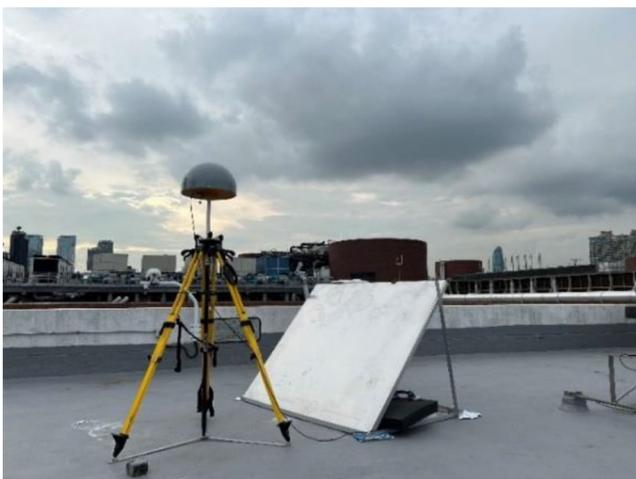
**Fig. 1** Experimental setup for below-antenna multipath data collection. A steel panel was used to generate controlled and strong reflected signals at the rover antenna
