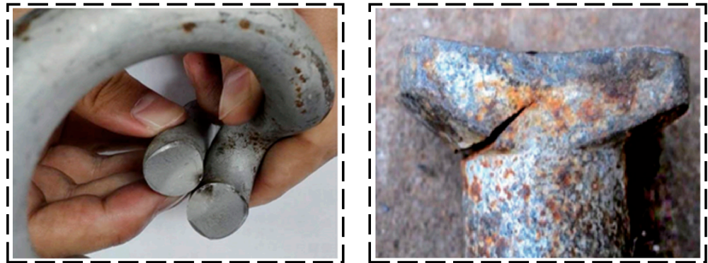
Figure 5. Secondary diseases caused by rail corrugation [34].
