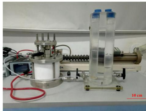
Fig. 2. The experimental device of the mock-up test: (a) Schematic view of the experimental device; (b) Photograph of the test system.
