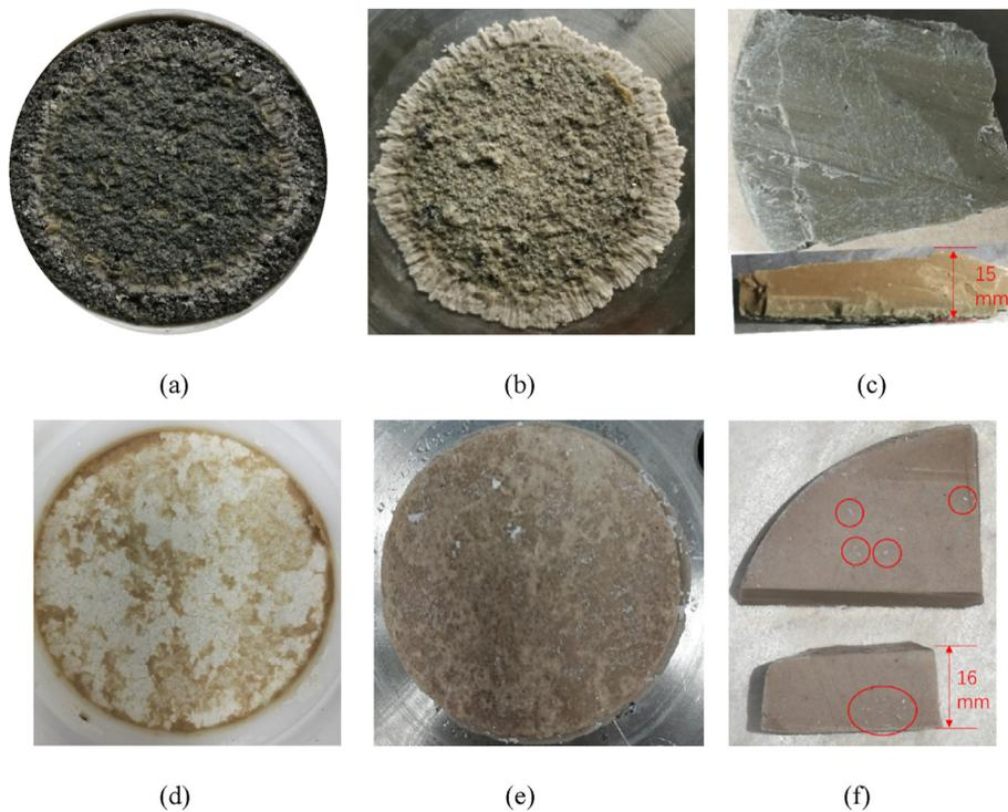
Fig. 4. The samples after mock-up tests. Sample #1: (a) Top surface of the concrete; (b) Bottom surface of the specimen; (c) Bottom and longitudinal sections. Sample #3: (d) Top surface of the concrete; (e) Bottom surface of the specimen; (f) Bottom and longitudinal sections.
