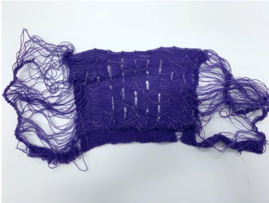
Figure 7. Knitted POF sample without support yarn.
