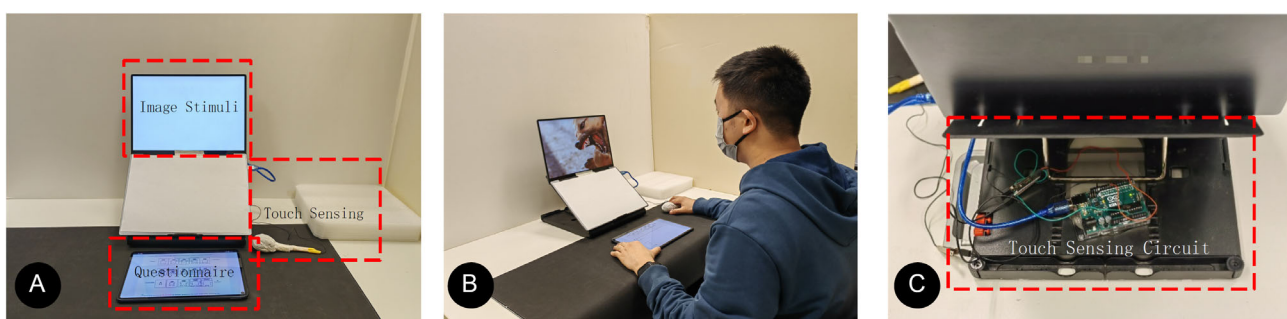
Figure 8. Experimental layout: A) Image stimuli are shown on the laptop screen, a touch-sensing model is adopted to capture participants' MGs, and a tablet is used to answer the questionnaire. B) We show how participants interact with our devices. C) The touching-sensing circuit based on the Arduino board is hidden behind the laptop.
