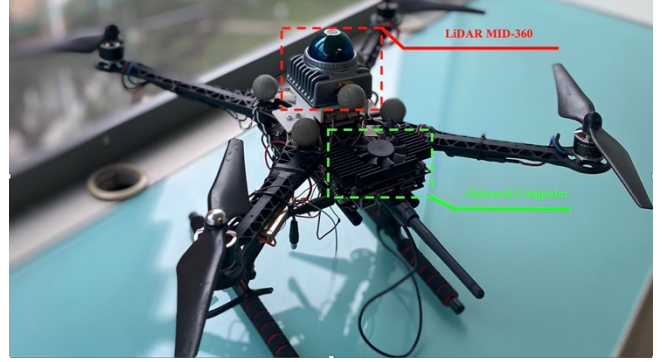
Fig. 11. The UAV with a LiDAR MID-360.
