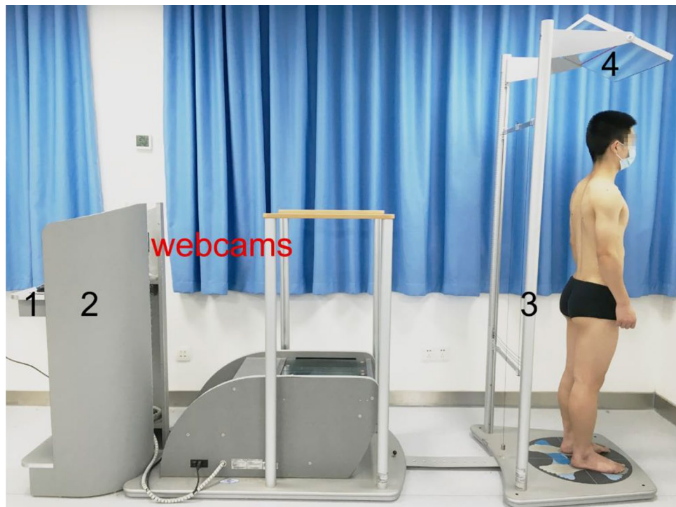
Figure 1. Set-up of recording digital images of participants' whole body via the 2D photogrammetry method using the GPS 400 posture evaluation system.
