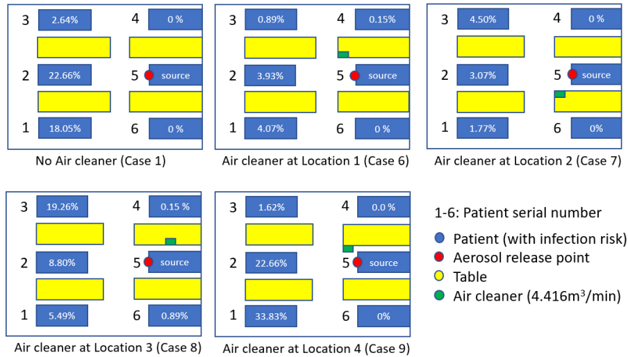
Fig. 10 The results of the infection risks of the six patients under CADR of 4.416 m³/min
