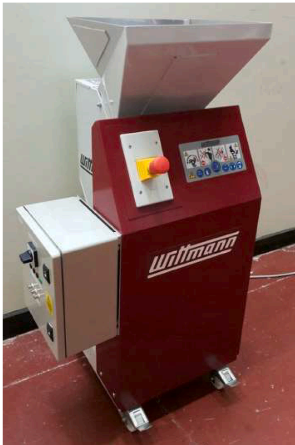
Fig. 5. Mechanical MAS1 Wittmann granulator recycling machine. Reproduced with permission from Elsevier [37].
