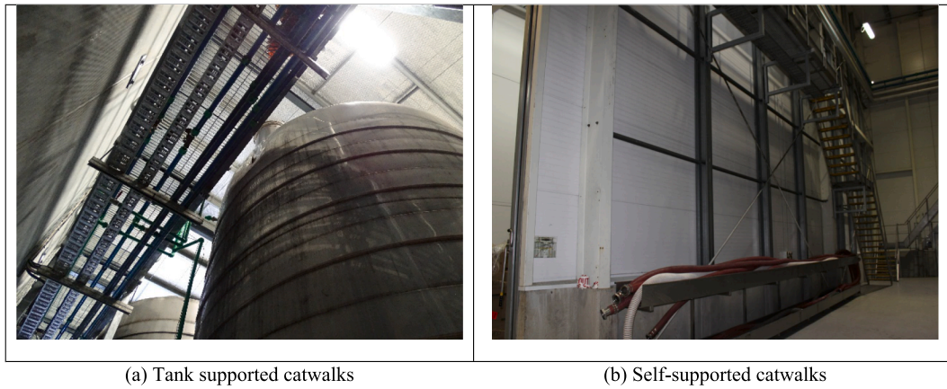
Fig. 2. Catwalk types commonly used in the wineries.
