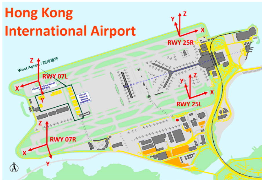
Fig. 11. Coordinate system transformation for HKIA.
