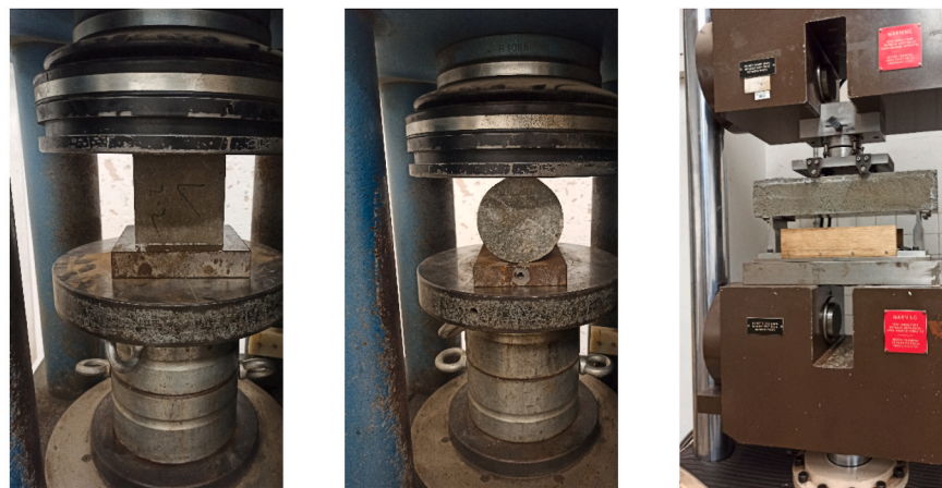
(a) Compressive strength test setup (b) Splitting tensile strength test setup (c) Flexural tensile strength test setup
