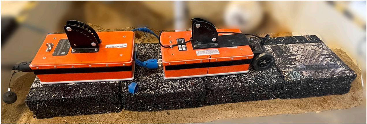
Fig. 6. Laboratory GPR measurement setup.
