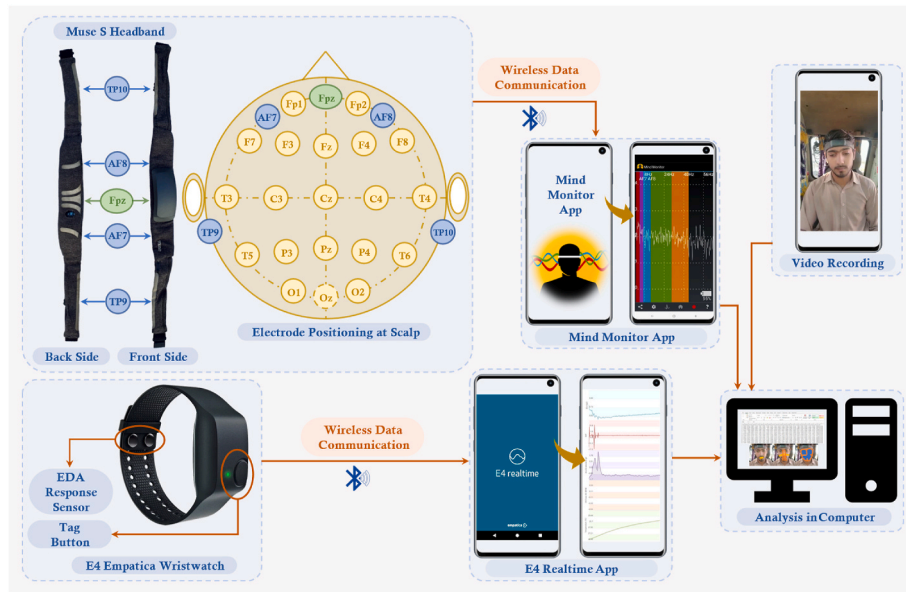
Fig. 3. Overview of apparatus utilized to collect and transfer the acquired data.
