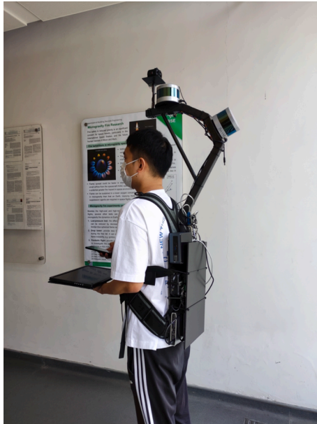
Fig. 3. The SLAM system in this study for dataset generation.
