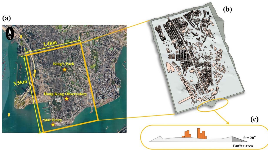
Fig. 6. Study area for CityFFD simulation: (a) plane view of the target area (where weather stations are marked with stars), (b) geometries of buildings and terrain, (c) setting of buffer areas.
