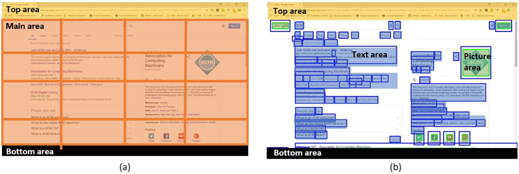
Fig. 9. Dynamic-UI Component Detection Methods: (a) Heuristic-based, (b) Content-based.
