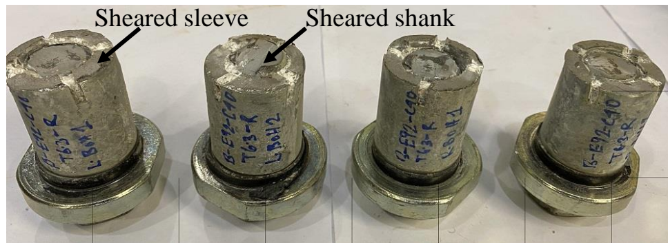
(c) Blind-bolts after failure in specimen B-E92-C40-T6.3-R
