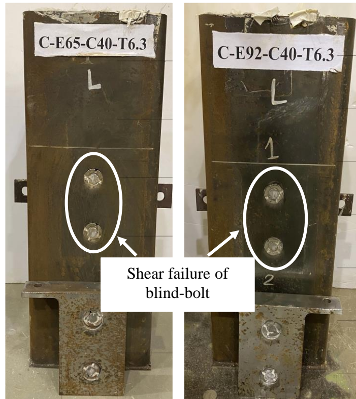
Figure 10: Specimens in series C after testing.
