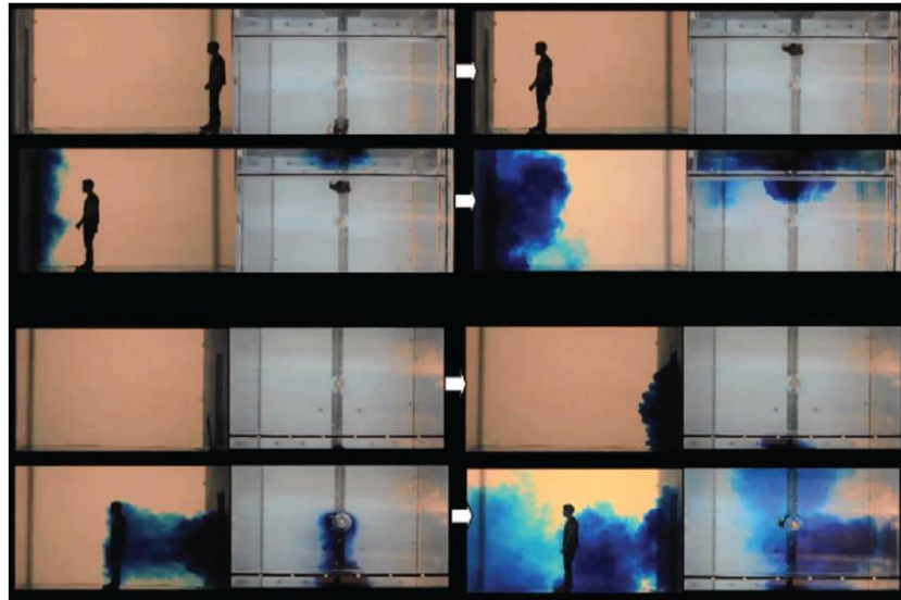
Figure 8. Snapshots of food dye movement due to door-opening motions and actions of the manikin. 120
