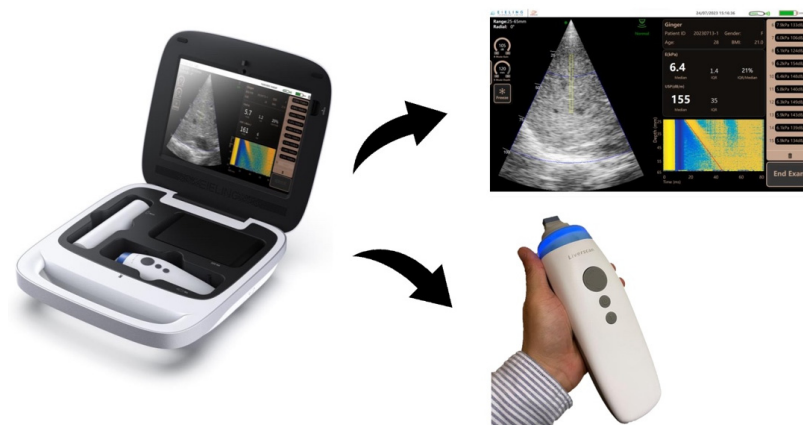
Figure 1. Schematic diagram of the Liverscan probe and paired software interface. Working principle of the Liverscan system: LSM procedure including shear wave generation and ultrasound acquisition is guided by real-time B-mode imaging. The displacements of the elastic liver tissue caused by the passage of the shear wave are documented via ultra-fast RF acquisitions, resulting in the formation of an elastogram. The elastogram, which estimates the Young’s modulus of the liver, is visualized as a strain image as a function of time and depth.
