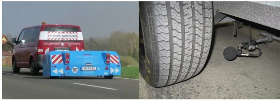
Fig. 15. CPX-trailer supplied by Müller-BBM (left) and standardized tire with measurement microphones in the anterior position (right) (Villaret et al, 2021).
