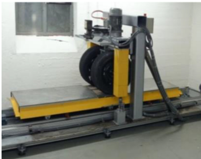
Fig. 20. The Aachen polishing machine (APM) (Wang et al, 2014).
