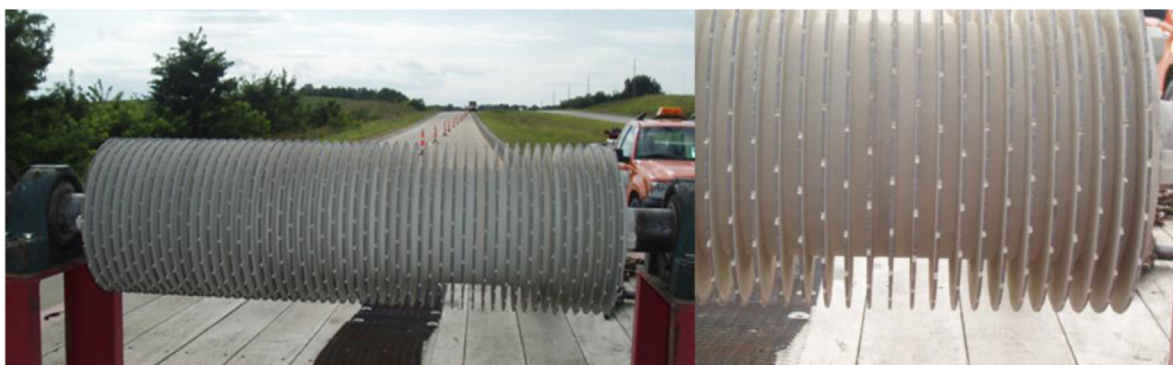
Fig. 6. Pictures of the grooving shaft (Cable and Wiegand, 2010).
