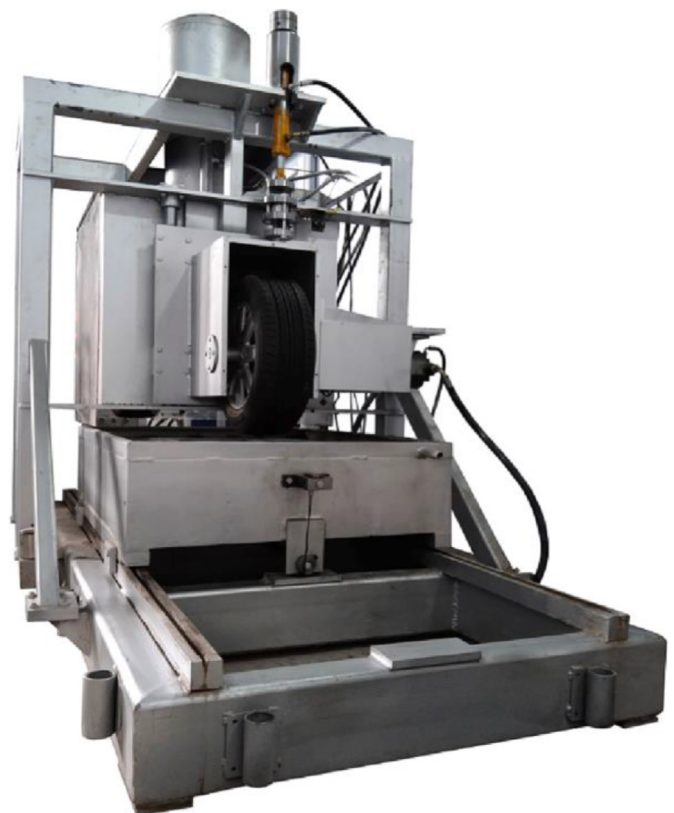
Fig. 13. The Harbin high-speed friction testing equipment.
