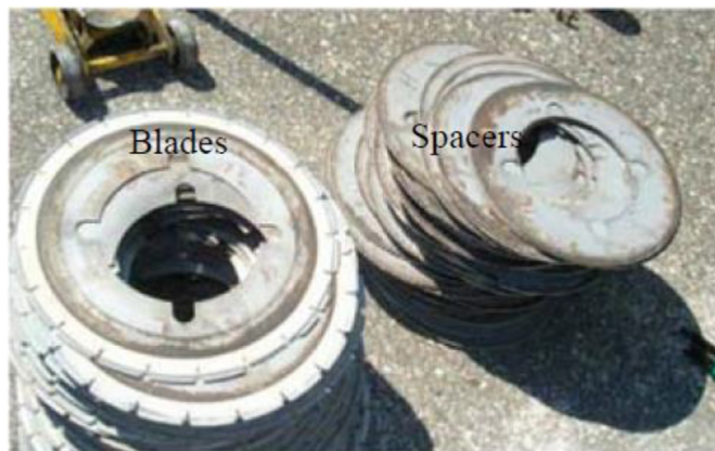
Fig. 3. Diamond grinding wheel with spacer wheel (Izevbekhai and Khazanovich, 2013).
