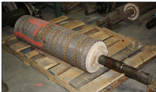
Fig. 2. Grinding shaft of 1.2 m in width (Villaret et al, 2021).
