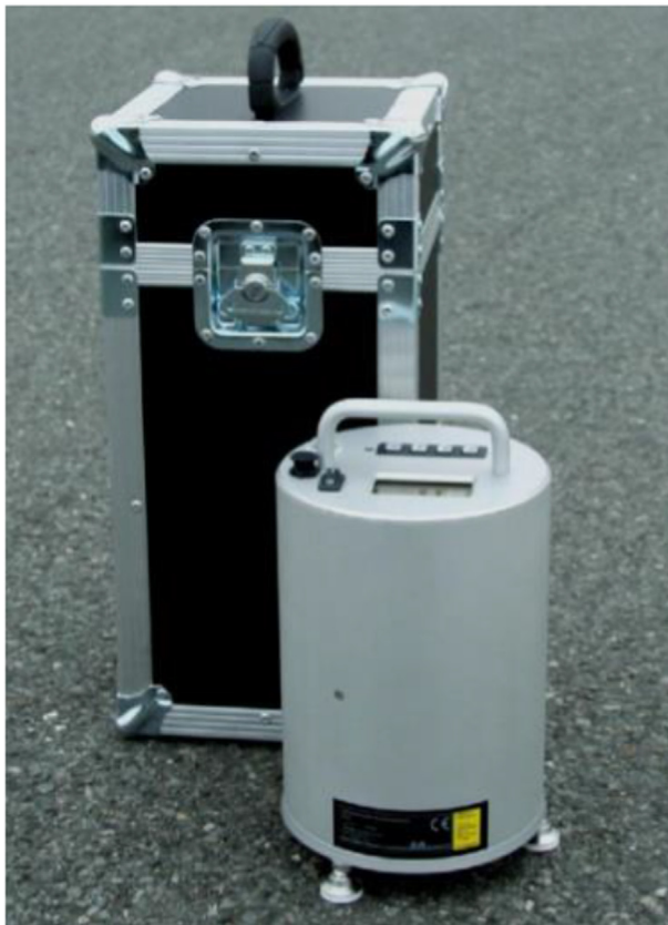
Fig. 9. MPD measurement of the optical method using ELAtextur.
