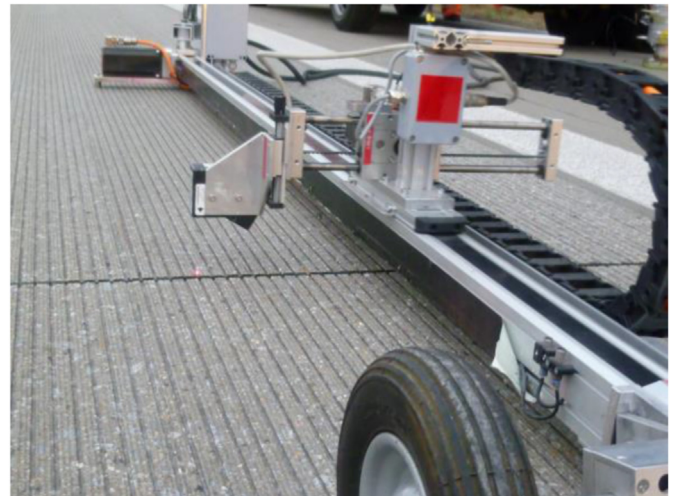
Fig. 11. Laser profilometer during field investigation (Villaret et al, 2021).
