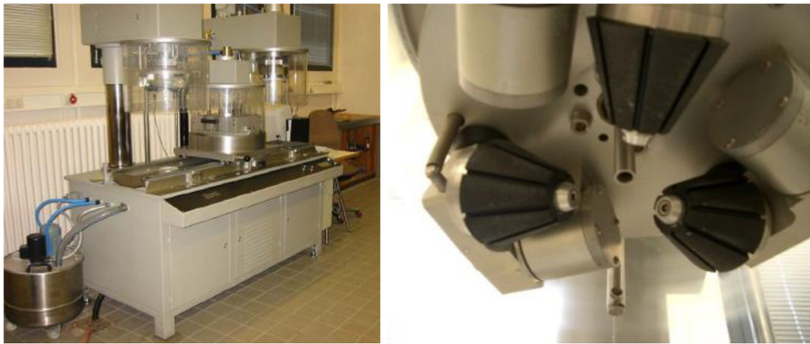
Fig. 12. The Wehner/Schulze (W/S) test machine (Wang et al., 2018).
