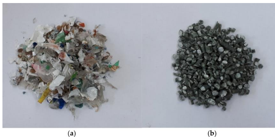
Figure 4 Appearance of plasmix (a) shreds before extrusion (b) pellets after extrusion and granulation (Celauro et al., 2021)
