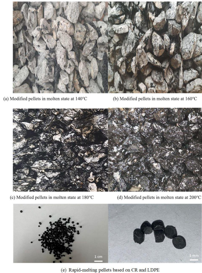
Figure 12 Rapid-melting pellets based on CR and LDPE composite (T. Liu et al., 2022; C. Zhao et al., 2023)
