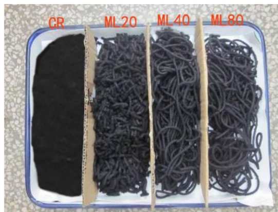
Figure 24 Devulcanized CR of different extrusion temperatures
