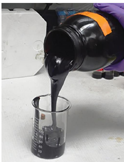
Figure 25 Liquid rubber prepared by vacuum pyrolysis (Fini et al., 2016)
