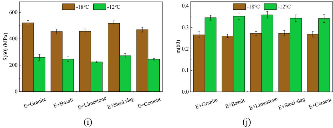
384 **Figure 7.** BBR test results of asphalt mastics: (a)  $S$  of A; (b)  $m$ -value of A; (c)  $S$  of B; (d)
