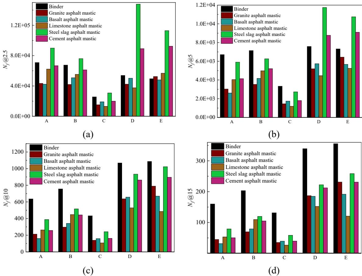
367 **Figure 6.** The fatigue life of asphalt mastics at different strain levels of (a) 2.5%; (b) 5%; (c)
