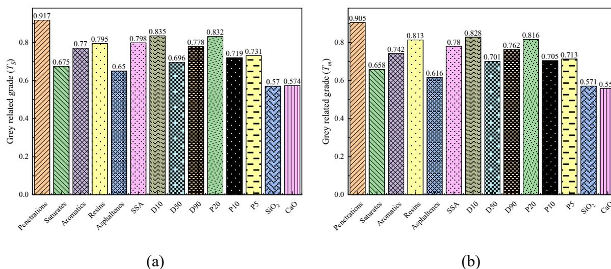
451 **Figure 11.** Grey relational grades between the low-temperature indexes and the raw material
