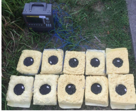
Fig. 1. Specimens for outdoor solar radiation test.
