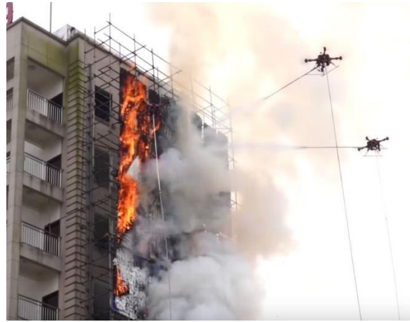
Figure 3. A demonstration for using multiple UAVs to suppress exterior façade fires on a structure [63].
