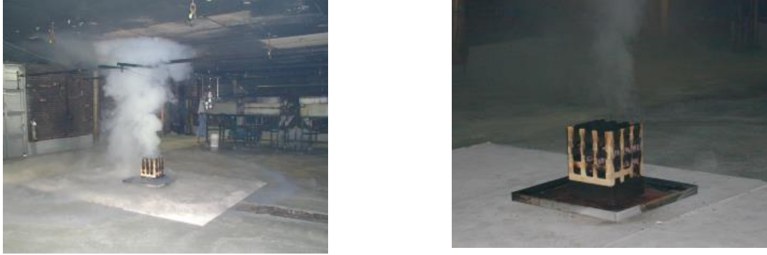
Figure 5. Extinguishment of wood crib fires by one liter of liquid nitrogen. In some of the tests the wood crib kept smoldering and slowly reignited after flame extinguishment [77].
