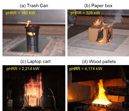
Fig. 1. Typical burning items in the NIST Fire Calorimetry Database. (a) trash can, (b) paper box, (c) laptop cart, and (d) wood pallets.
