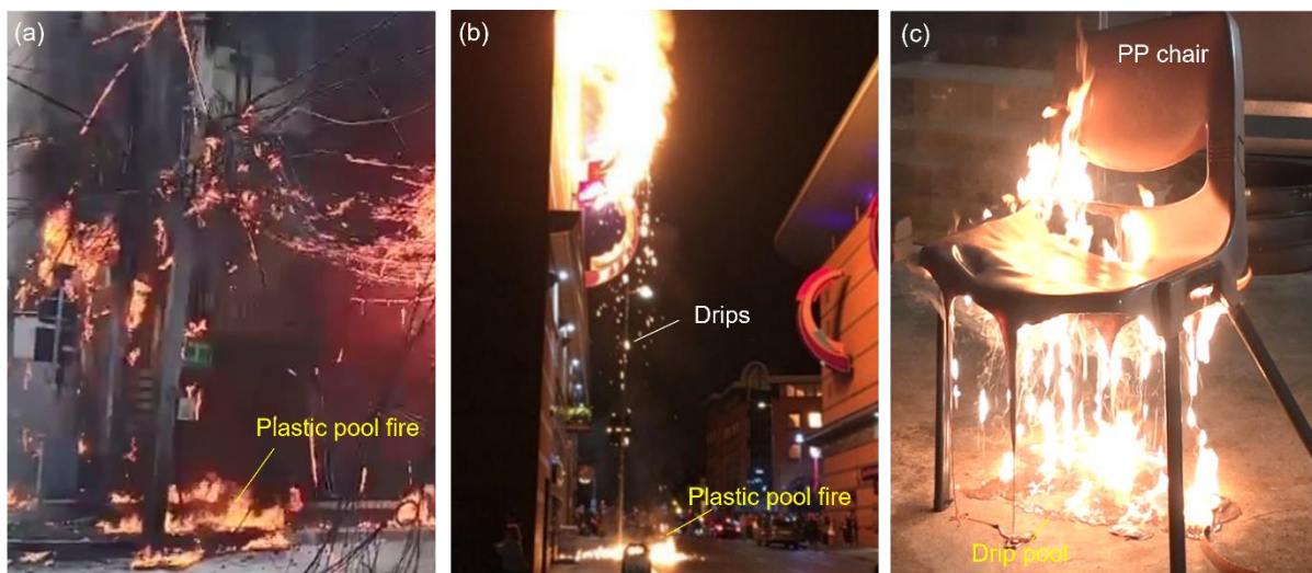
Fig. 1. (a) Plastic pool fire in a real cable fire accident [21] (b) The plastic advertising light caught fire and formed a drip pool at ground [22], and (c) pooling of burning PP chair.
