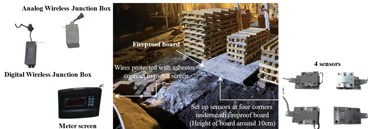
Fig. 5. The set-up of weighing scale (XK3190-AW1).
