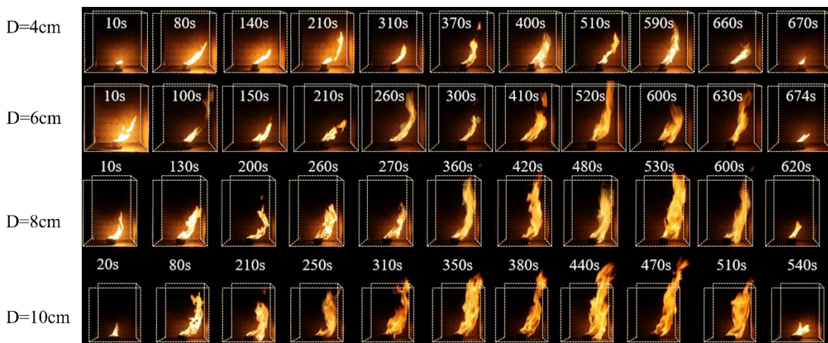
Fig. 2. Flame evolution of pool fire inside semi-confined compartment under the cross wind velocity of 1.71m/s
