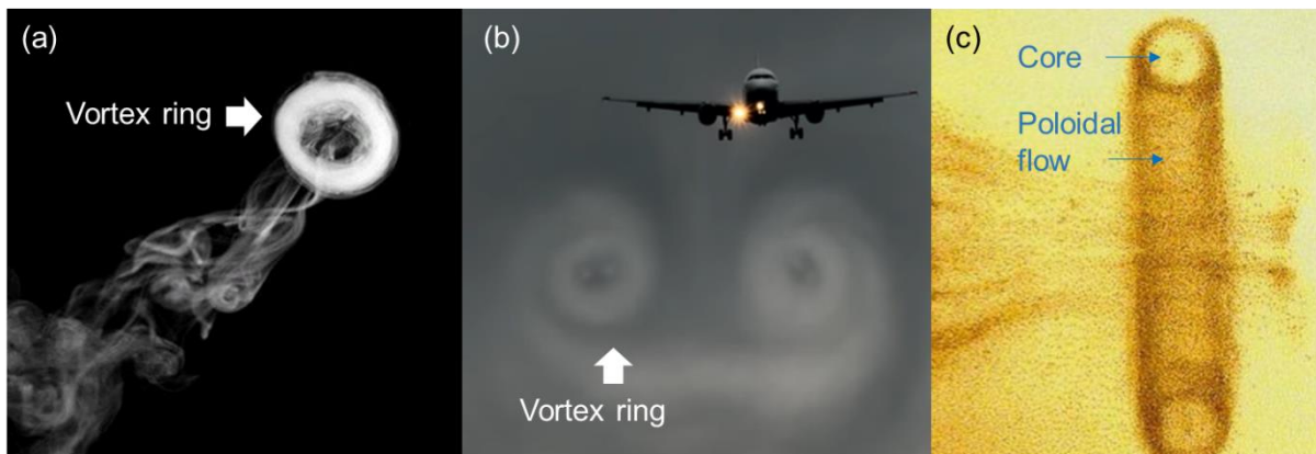
Fig. 1. (a) Smoke vortex ring [26], (b) gas vortex ring [27], and (c) sectional view of air vortex ring [28].
