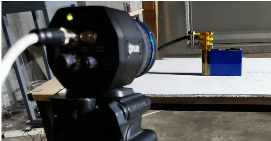
Fig. 4. Tab heating infrared thermography experimental setup.
