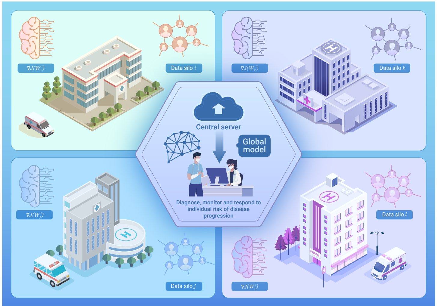
Figure 9. Schematic of federated learning. In a multi-party collaboration, to preserve the privacy of data, federated learning only allows remote devices to exchange model gradients with a central server. During this process, each distributed model is trained only using local data, and then the computed gradients are uploaded to the central server. Subsequently, the central server updates the global model based on the collected gradients and sends back the updated parameters of the global model. Finally, the well-trained global model applies for different locations and data sources.
