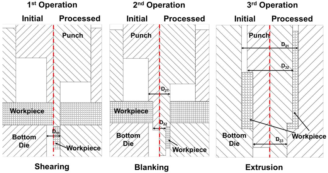
**Figure. 3.** Improved three-stage forming system based on extrusion.
