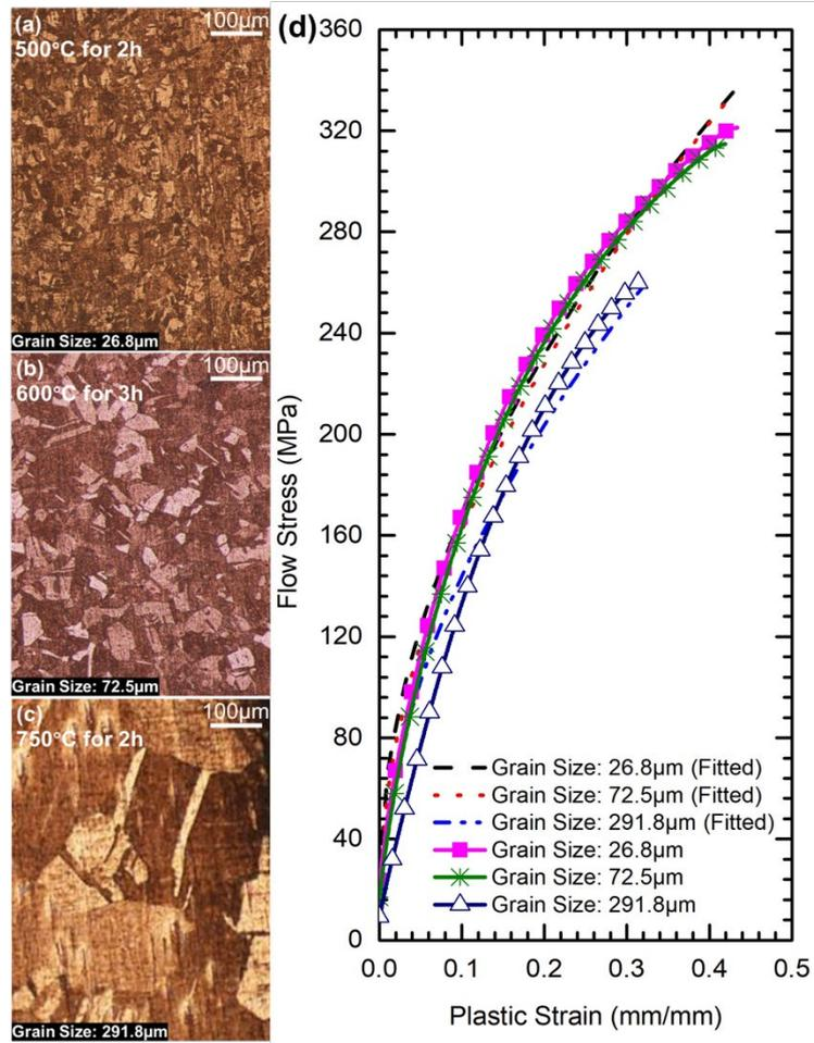
**Figure. 1.** Microstructures of pure copper annealed in various conditions: (a) 500°C for 2h, (b) 600°C for 3h, and (c) 750°C for 2h; (d) properties of materials with various grain sizes (GSs).
