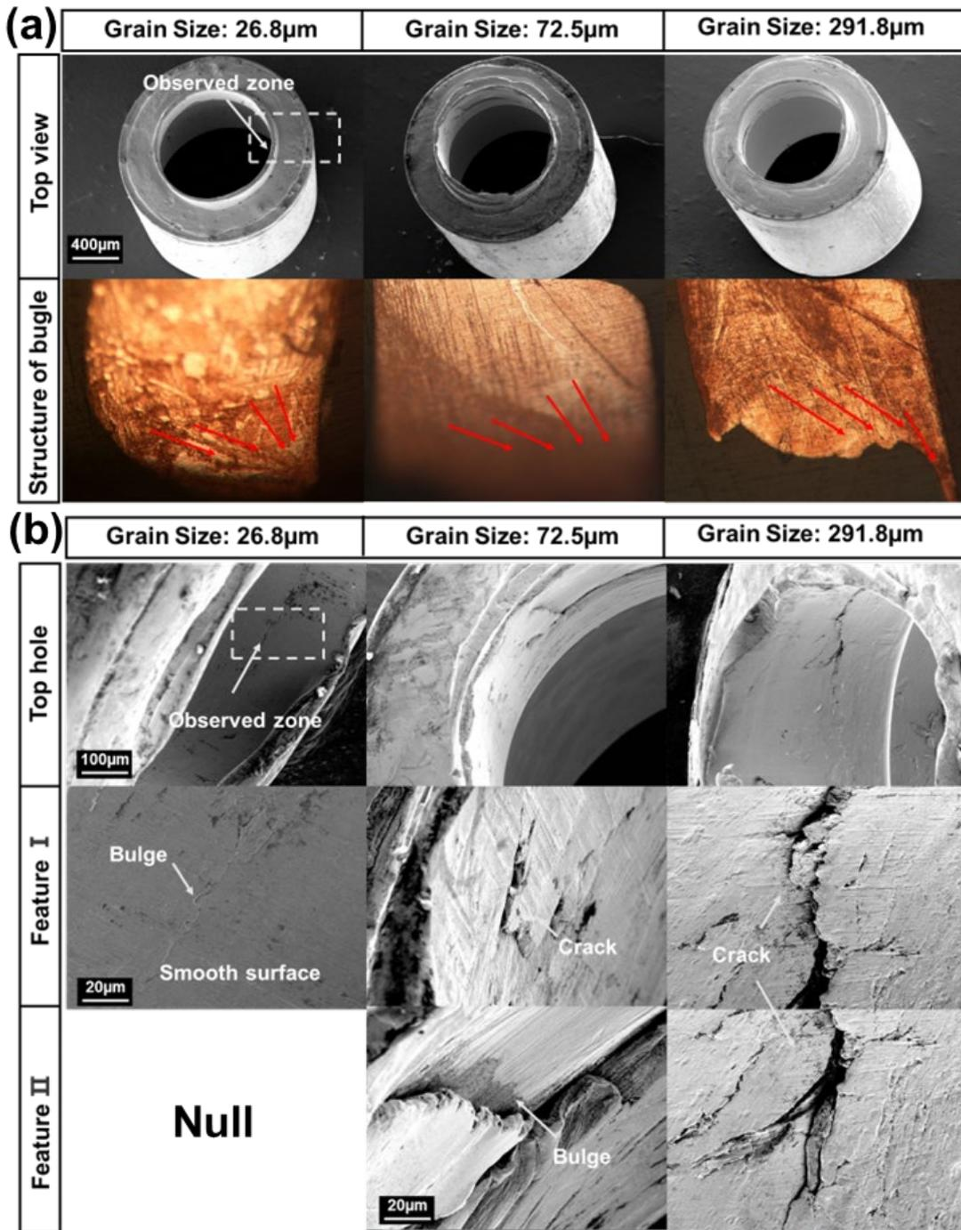
**Figure. 12.** SEM images: (a) external surfaces of the top holes and (b) internal surfaces of the top holes.
