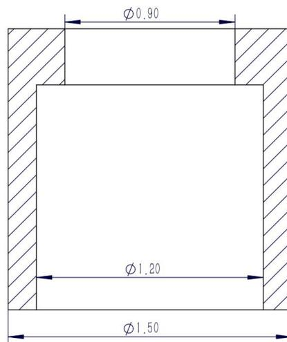
**Figure. 2.** Dimensional schematic of the target part (Unit: mm).
