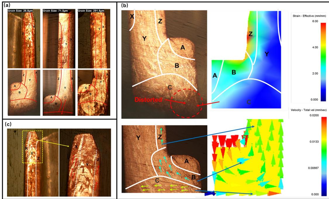
**Figure 6.** (a) Microstructural evolutions of components with various GSs; microstructural evolution of the components annealed at 500°C for 2 h: (b) metallographic microstructures, distribution map of strain and flow velocity in top hole area, (c) metallographic microstructures and strain distribution in earing area.
