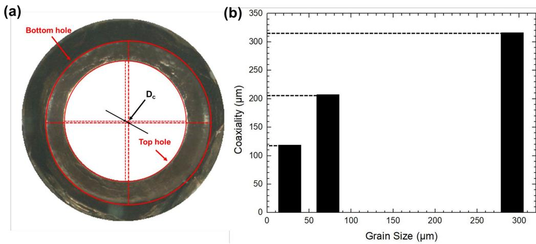
**Figure. 9.** (a) Diagrammatic representation of the coaxiality, (b) coaxiality of the bottom hole.
