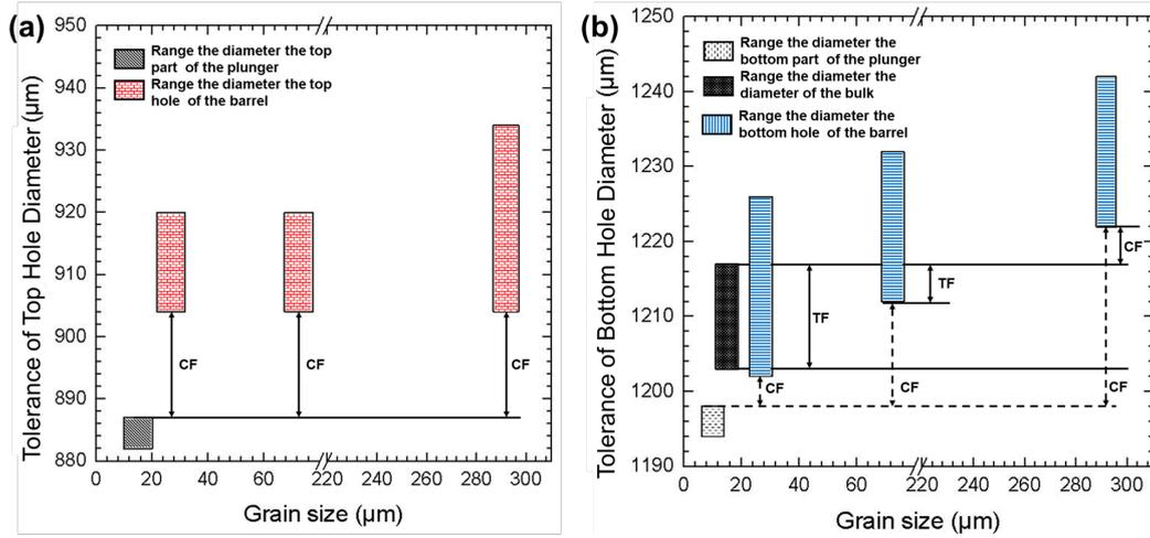
**Figure. 8.** Assembly conditions: (a) conditions of the top hole, (b) conditions of the bottom hole.
