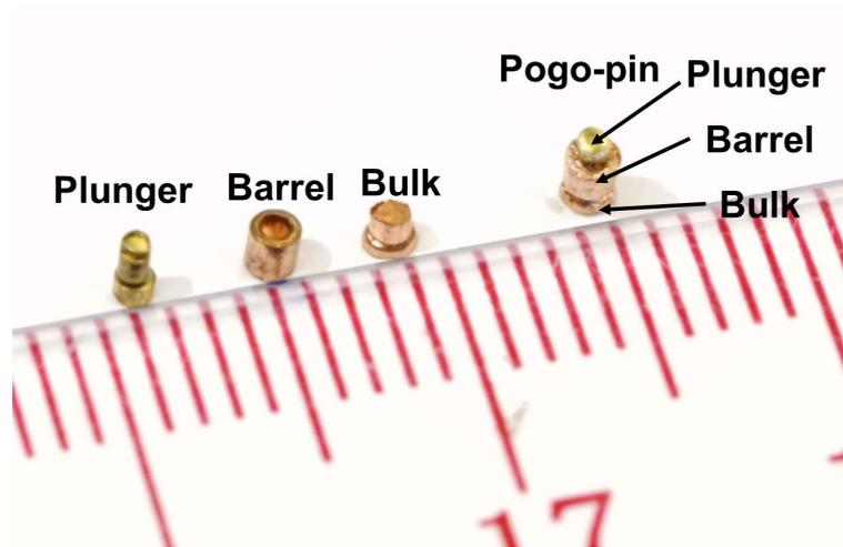
**Figure. 10.** Assembled pogo-pin and corresponding parts.
