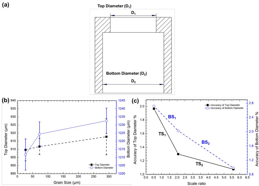
**Figure 7.** (a) Diagrammatic representation of the measured diameter, (b) diameter of the top hole ( $D_1$ ) and diameter of the bottom hole ( $D_2$ ), and (c) accuracy of both holes with various scale ratios.
