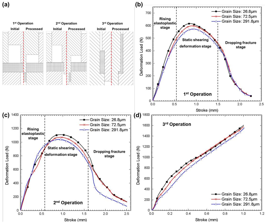
**Figure 4.** (a) Schematic diagram of each operation, and load-stroke curves in (b) the first operation, (c) the second operation, (d) the third operation.
