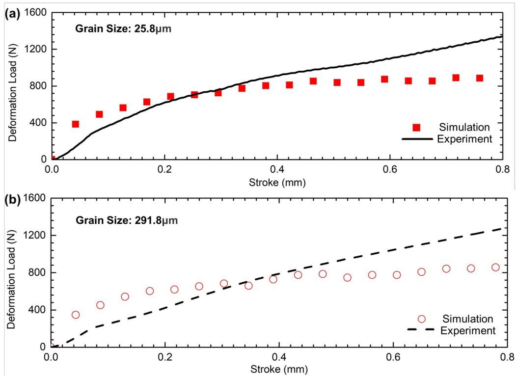
**Figure 5.** Comparison of stroke load curves obtained by simulations and experiments with various GSs: (a) 25.8 μm and (b) 291.8 μm.
