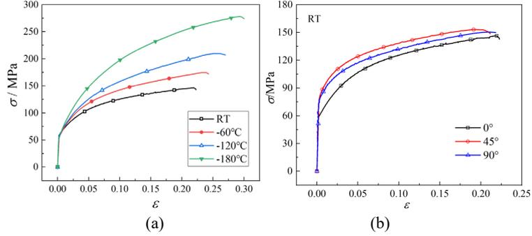
**Fig. 1.** True stress-strain curves obtained by uniaxial tension tests: (a) 0° tension at different temperatures, (b) 0°, 45° and 90° tension at RT.
