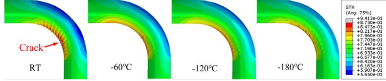
Fig. 4. The FE simulation results of the thin-walled 6061-O aluminum alloy tube bending.
