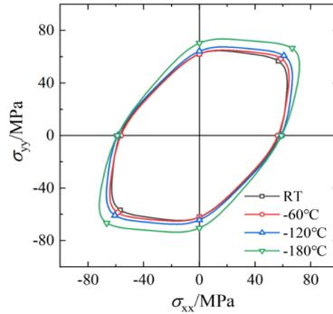
**Fig. 2.** The yield locus of the thin-walled 6061-O aluminum tube at different temperatures.
