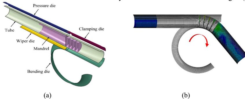
**Fig. 3.** FE model establishment: (a) geometry model, (b) rotary draw bending FE model.
