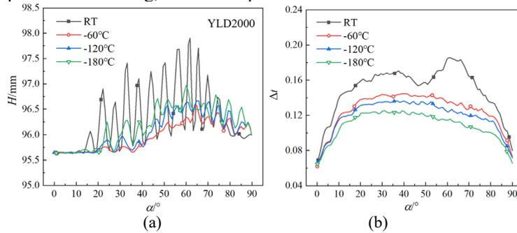
Fig. 5. Forming defects of the tube at different temperatures:(a) wrinkling pattern along tube inner ridgeline, (b) wall thickness reduction rate along tube outer ridgeline.
