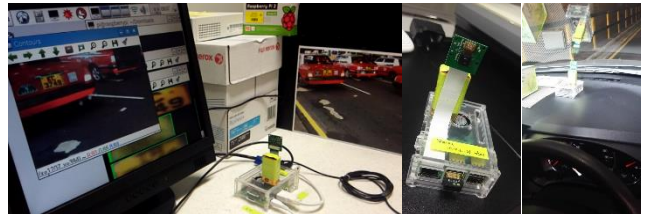
Fig. 7. Implement LPR system in RPI.
