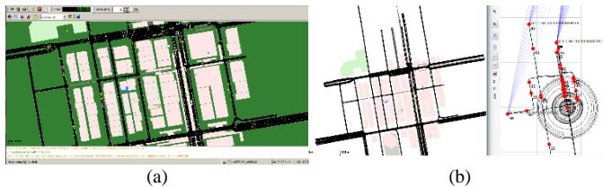
Fig. 2. VANET scenario construction in both SUMO and NS-3
