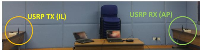
Fig. 2. NLOS scenario setup with 2 USRP N210 antenna modules
