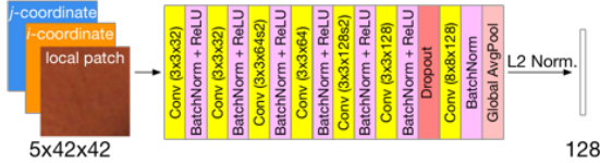
Fig. 2: The network architecture of PoreNet, adapted from HardNet [11]. Each skin patch is concatenated with the i -coordinate and the j -coordinate channels, corresponding to the (x, y) coordinates, as the input. Stride of 2 is denoted as s2 .
