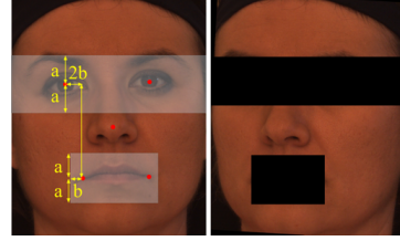
Fig. 4: Illustration of the measurement of the occluded regions (left), and occluded regions of a query image (right).
