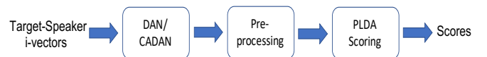
Fig. 2: Transformation of i-vectors by the feature extractor of DAN or CADAN and pre-processing for PLDA scoring. The transformation is considered as domain adaptation in this work.
