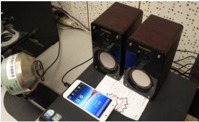
Fig. 7. The setup for recording the station-noise contaminated sound events. The mount simulator on the left are used for playing the sound events and the two speakers in the middle are for playing the station noise. The sound events and station noise are added acoustically and recorded by the mobile phone in the middle.
