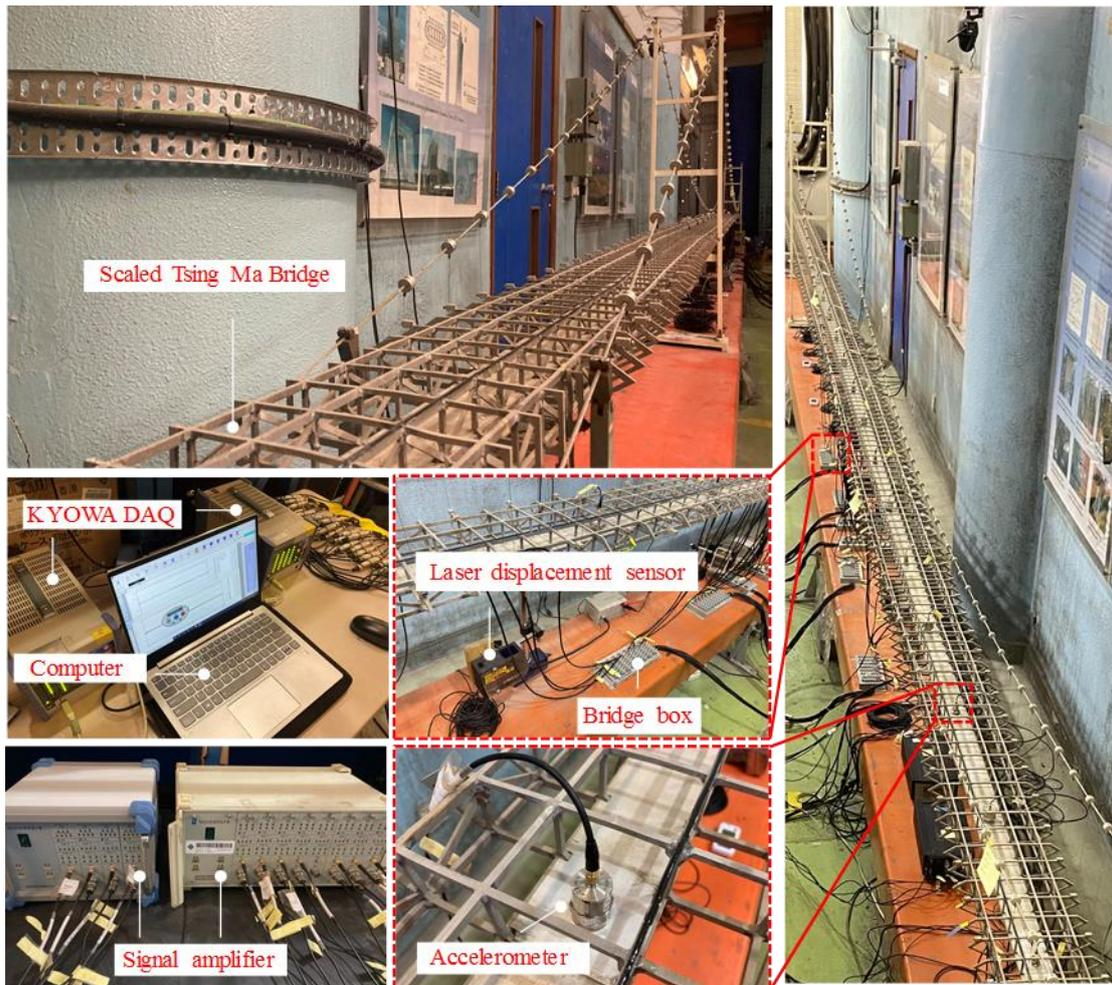
Fig. 4 Photograph of the experimental setup
