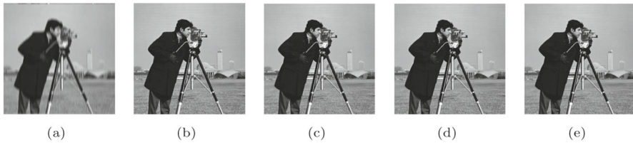
Fig. 2 Nonconvex image restoration. Recovered images with the three solvers for \epsilon_0 = 10^{-3} and \lambda = 10^{-2} . a Noisy blurred image, b original image, c IRPNM, d ZeroFPR, e GIPN-F
