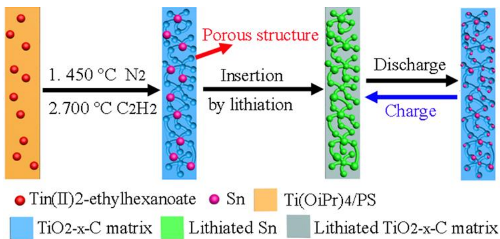
Figure 1. Schematic illustration of the formation of highly stable porous \text{TiO}_{2-x}\text{-C-Sn} composite nanofibers and insertion of Sn nanoparticles.
