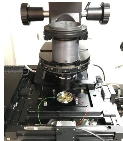
Fig. 3 Experimental setup for DEP cell patterning onto the scaffold
